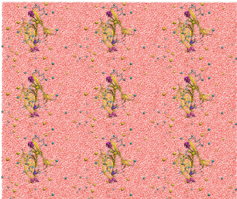
Fig. 10.1 Illustration of the periodic boundary conditions in two dimensions. The graph is produced using VMD program (Humphrey et al. 1996)
